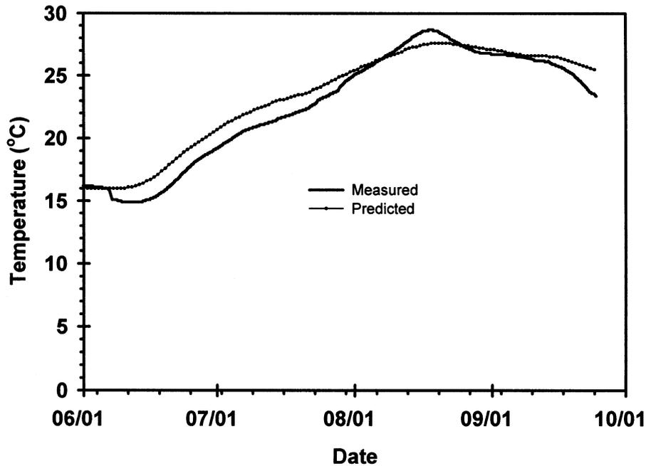
Figure 2. Measured and predicted temperatures 0.7 m from the plenum floor in the center of non-aerated bin 9 during the 2001 storage season when the model was solved using the predicted natural convection currents with a sealed plenum.
