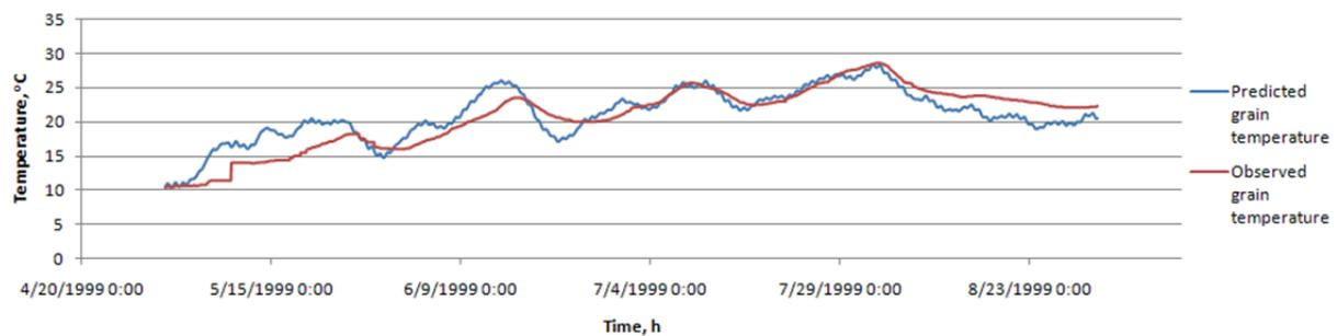
Figure 4. Grain temperature 0.9 m above the plenum near the center of the grain mass in PHERC Bin 12 during May-August 1999 for Q-1.
