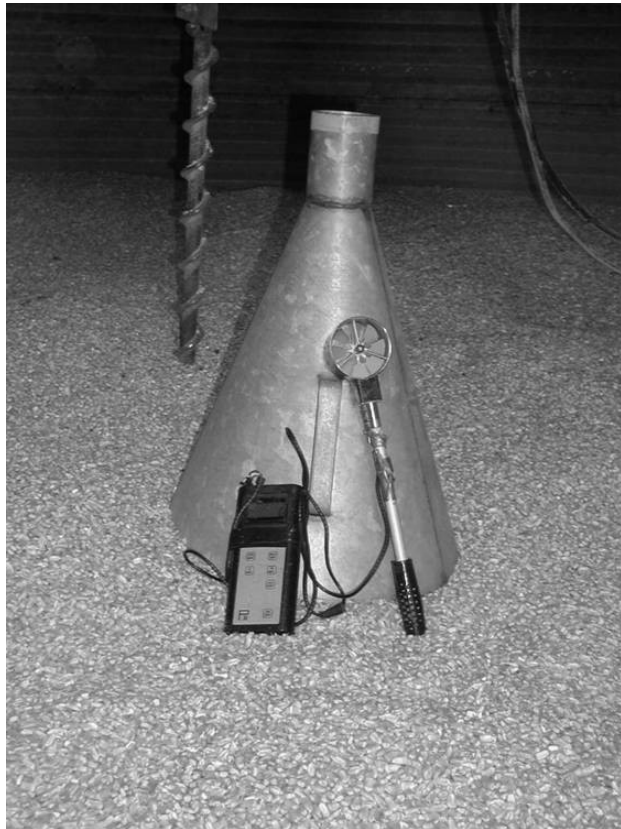
Figure 2. Funnel and anemometer used for measuring air velocity at different grain surface locations in the bin for natural air / low temperature in-bin drying and conditioning experiments.
