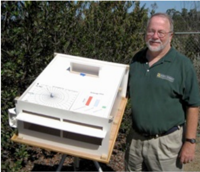
The solar simulator being used for a south wall daylighting and solar control evaluation
