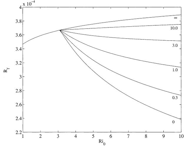
FIG. 3. Mixing efficiency computed from entrainment experiments as a function of the Richardson number for various values of the density ratio, shown below each curve. For  $Ri < Ri_c$ , heat and salt are entrained at equal rates.
