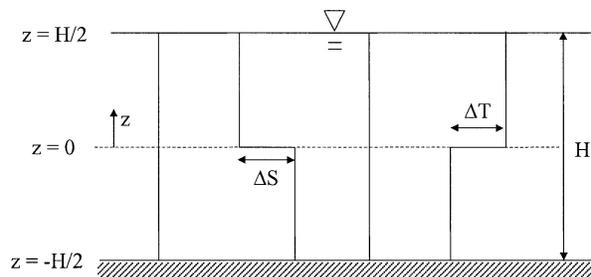
FIG. 1. Initial salinity and temperature profiles used in the models. The mean temperature and salinity are  $T_0$  and  $S_0$ , respectively, and the temperature and salinity differences,  $\Delta T$  and  $\Delta S$ , are taken to be positive. The length, width, and depth of the fluid are  $L$ ,  $B$ , and  $H$ , respectively.
