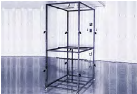
FIG 2 Steel frame with calibration markers (shown by arrows)
