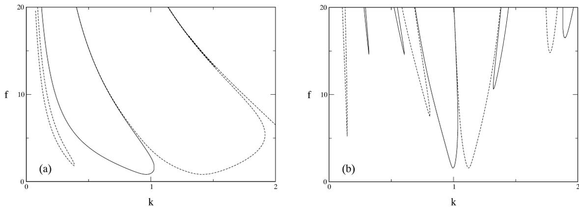
Fig. 4. Neutral stability curves computed from (20) linearized about  $h = \Phi = 0$ . Floquet multipliers of +1 (–1) are indicated by solid (dashed) lines. (a)  $m/n = \frac{2}{3}$ ,  $\phi = 0^\circ$ ,  $\chi = \chi_c = 66.6^\circ$ ,  $\Gamma_0 = 0.53$ ,  $G_0 = 0.47$  and  $\gamma = 0.09$  in (20) and (21). (b)  $m/n = \frac{6}{7}$ ,  $\phi = 0^\circ$ ,  $\chi = \chi_c = 53.0^\circ$ ,  $\Gamma_0 = 7.5$ ,  $G_0 = 1.5$  and  $\gamma = 0.08$ .
