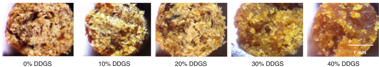
Fig. 4 Cross-sections of the resulting extrudates (magnification of \times 60 )
