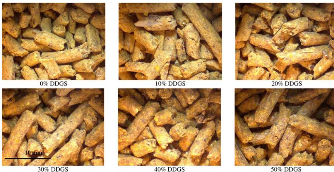
**Fig. 1.** Extrudates produced in this study were cylindrical in shape.
