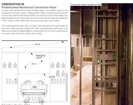
Figure 5: Field Report Showing Prefabricated Patient Room Mechanical Connection Panels. Students noted that, due to the IPD method, this cost-saving solution was proposed by subcontractors. (Andrew Shea 2014)
