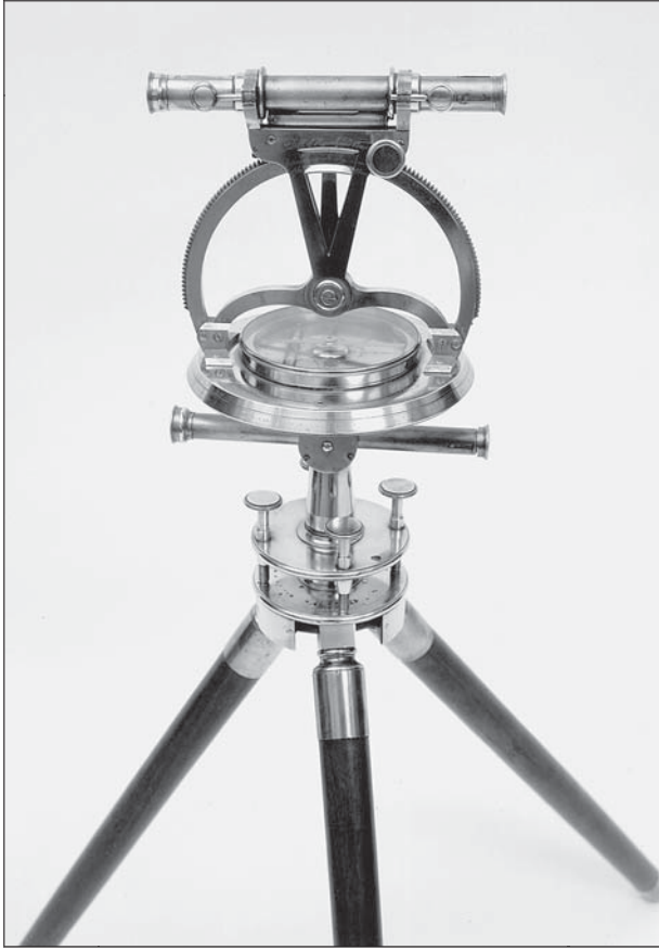
A theodolite is a survey instrument used to accurately map topography and property lines. Thomas Jefferson's theodolite, pictured here, is preserved at Monticello. Jefferson learned surveying in his youth and continued to use his skills throughout his life, mapping and measuring properties in Virginia.
