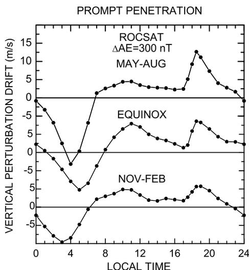
**Figure 1.** Seasonal dependence of longitudinally averaged equatorial prompt penetration vertical plasma drifts (positive upward) from ROCSAT-1 following a step function increase in the  $AE$  index by 300 nT.
