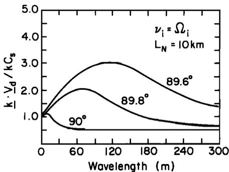
Fig. 8. Variation of the threshold drift velocity with wavelength and aspect angle at 122 km for  $2\alpha N_0 = 0.04 \text{ s}^{-1}$ . These results are not accurate for wavelengths smaller than about 20 m.
