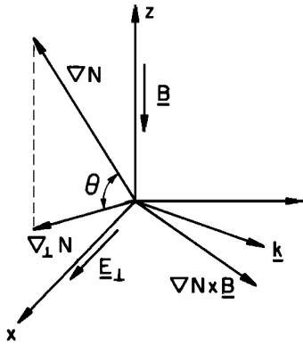
Fig. 1. Coordinate system used for the ambient electric and magnetic fields and electron density gradient. Here  $\nabla_{\perp}N$  is the density gradient component perpendicular to the magnetic field. For a horizontally stratified ionosphere the angle  $\theta$  between the ambient electron density gradient and the plane perpendicular to  $\mathbf{B}$  is the magnetic dip angle.
