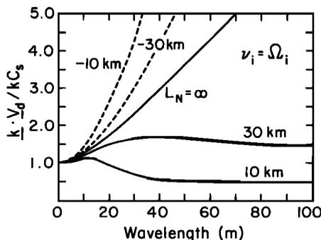
Fig. 6. Normalized threshold drift velocity for waves with  $\mathbf{k}$  perpendicular to the magnetic field at 122 km. The recombination rate  $2\alpha N_0$  was assumed to be  $0.04 \text{ s}^{-1}$ . These results are not accurate for wavelengths smaller than about 20 m.
