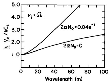
Fig. 5. Plot of the threshold drift velocity for waves propagating perpendicular to the magnetic field in a plasma with no electron density gradient at 122 km, where  $\Omega_i = v_i$ . These results are not accurate for wavelengths smaller than about 20 m.
