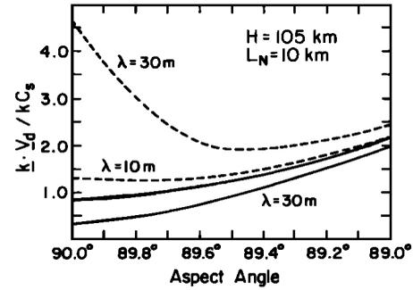
Fig. 3. Variation of the threshold drift velocity with aspect angle at 105 km with a recombination rate of  $0.06 \text{ s}^{-1}$ . The solid and dashed curves correspond to destabilizing and stabilizing electron density gradients, respectively.
