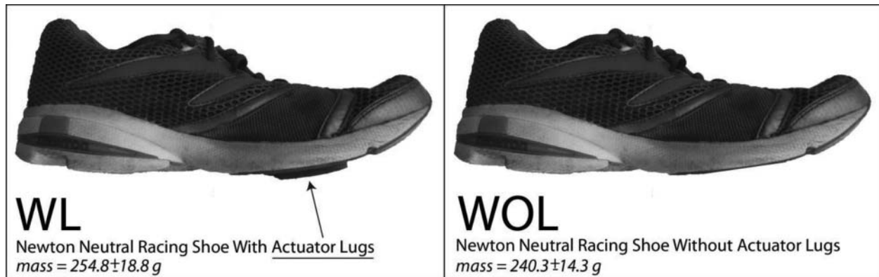
Figure 2. Two footwear conditions were used in this study (WL, WOL). The Newton Neutral Racer (WL; mass = 254.8 ± 18.8 g) was modified by removing the forefoot actuator lugs (WOL; mass 240.3 ± 14.3 g).
