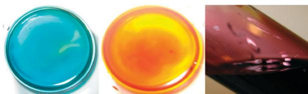
**Fig. 3** Dilute solutions (< 1 wt%) of sulfur (blue), selenium (orange) and tellurium (purple) in the ionic liquid  $[P_{6,6,6,14}][\text{decanoate}]$  at 50 °C (S, Se) and 170 °C (Te).
