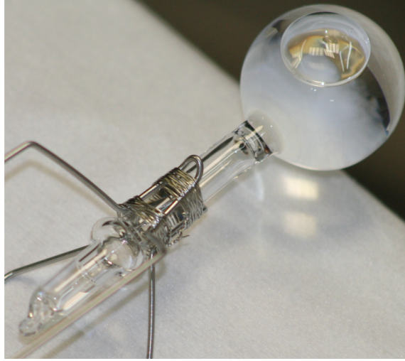
Figure 8. The ^{203}\text{Hg} \gamma source that was deployed in June, 2009. The spherical vial is made of quartz, whereas the neck is a graded transition from quartz to Pyrex. The rounded bulge in the neck is a safety feature to prevent the source from slipping out. Source retention is provided via the two independent wrappings with thin-gauge stainless steel wire.
