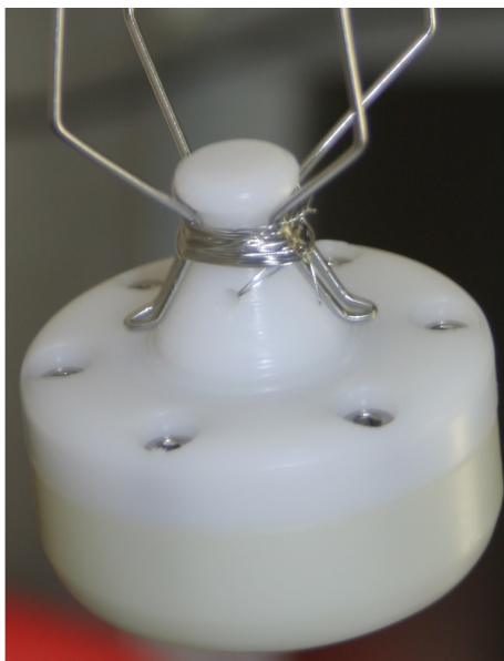
Figure 9. Photo of the encapsulation in which the Borexino ^{241}\text{Am}^9\text{Be} neutron source was placed. Note that the neck contains the same mounting features as the regular source vials.
