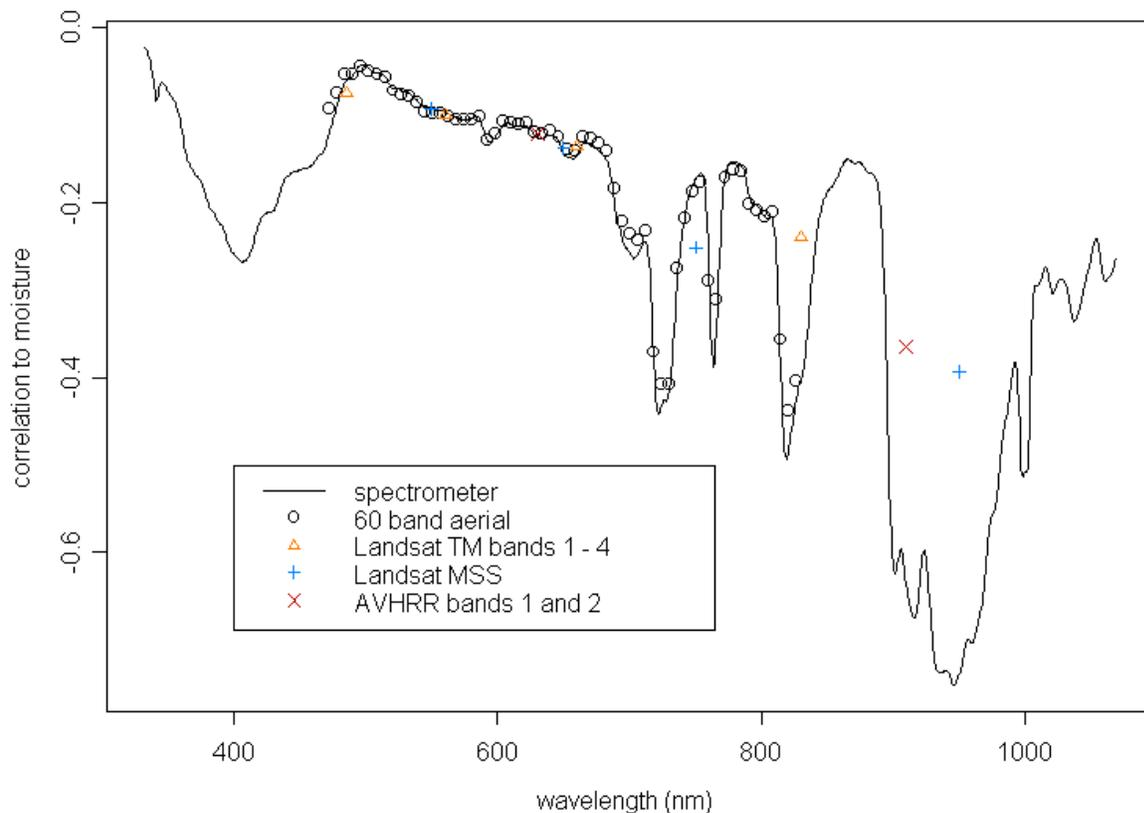
Figure 1. Correlation analysis for various spectral resolutions.
