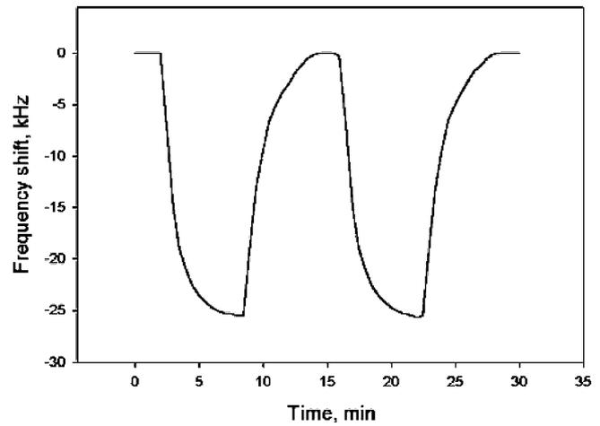
Fig. 3. TFPAS response (YAG substrate) to 100 ppm *n*-decane vapors under  $\lambda/4$  peak resonance.
