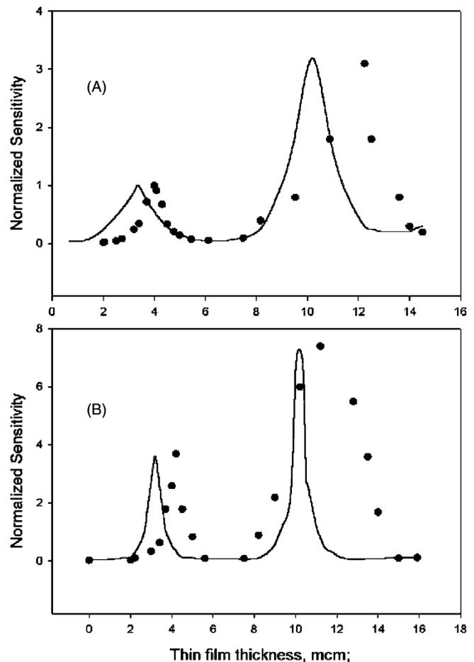
Fig. 4. Normalized (to  $\lambda/4$  resonance of fused quartz substrate) TFPAS sensitivity: (A) fused quartz substrate and (B) YAG substrate.
