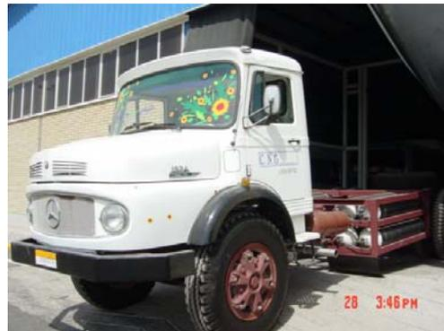
Clearly, for reinforcing the body with purpose of keeping the tanks and preventing concentration of tension in these points (because of increased weight), some modifications has been made on the body, chassis or different parts. In this system, different type tanks have been used side by side. Faber Company and MCS Company have made these tanks of steel or aluminum and reinforced them with composite fibers in radial direction .
