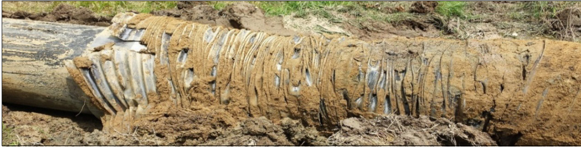
Figure 6: Folded CMP pushed out
