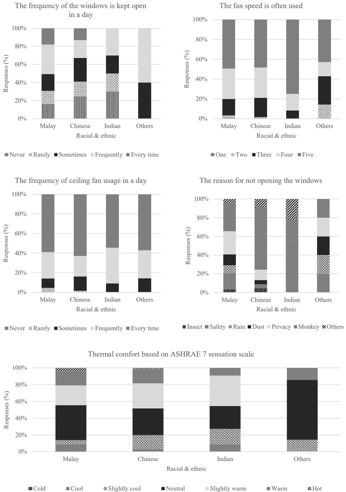
Figure 3: The usage pattern of windows, ceiling fan and the thermal comfort based on ASHRAE 7 sensation scale according to the racial and ethnic groups
