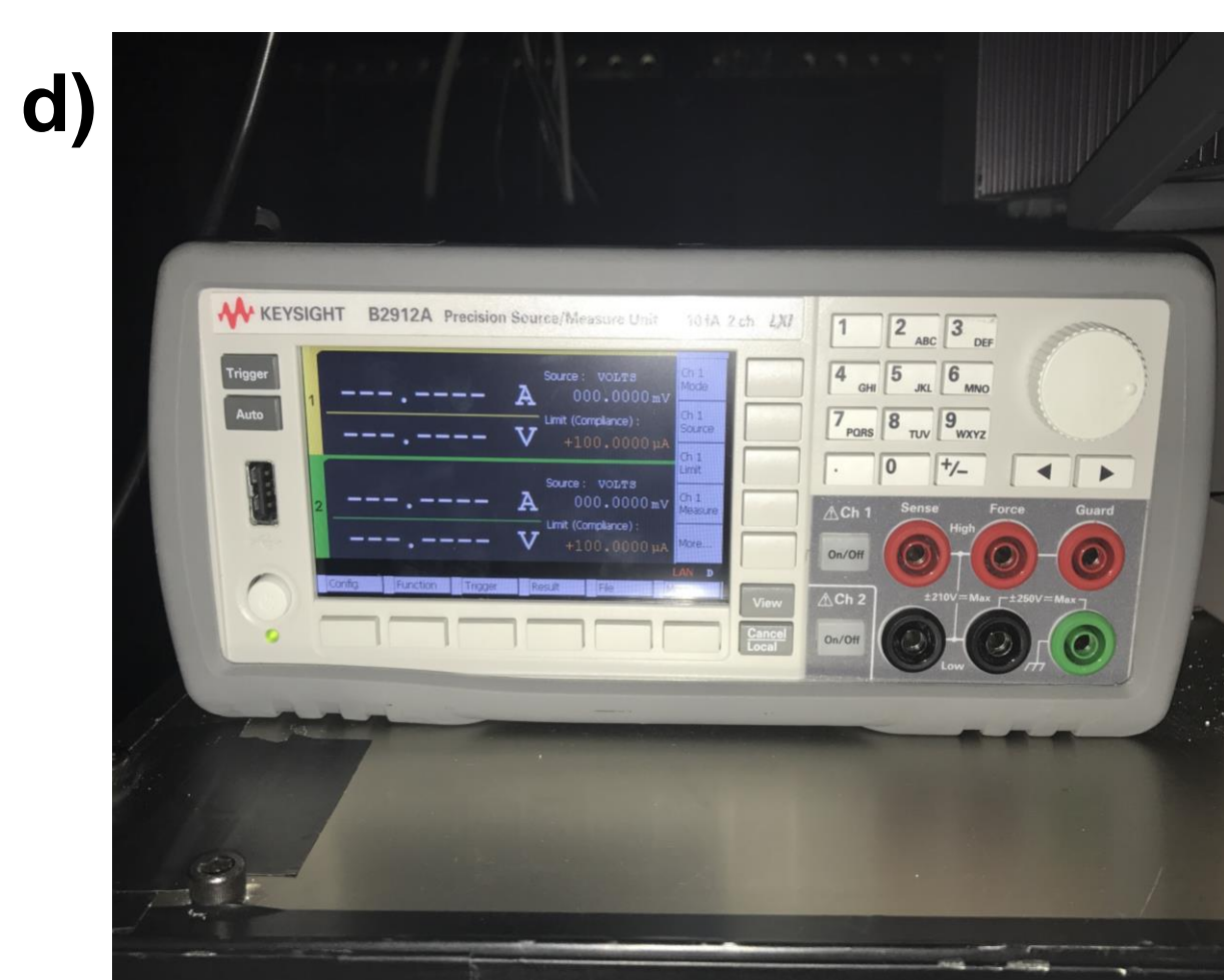
d. Keysight used for a DC Sweep (Lab View)
