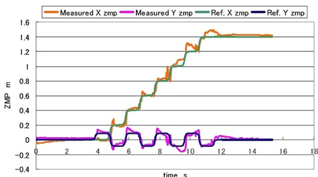
**Fig. 13** WABIAN-2R walked on the bumpy surface with tiles angled  $2^{\circ}$ – $5^{\circ}$  (forward-axis) down (experimental site no. 7)
