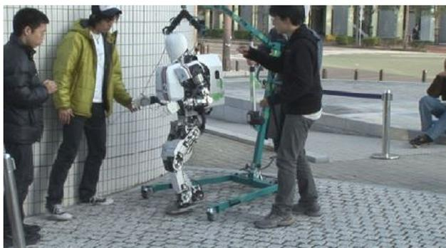
**Fig. 11** WABIAN-2R walked on the bumpy surface with tiles angled  $2^{\circ}$ – $5^{\circ}$  (forward-axis) down (experimental site no. 7)
