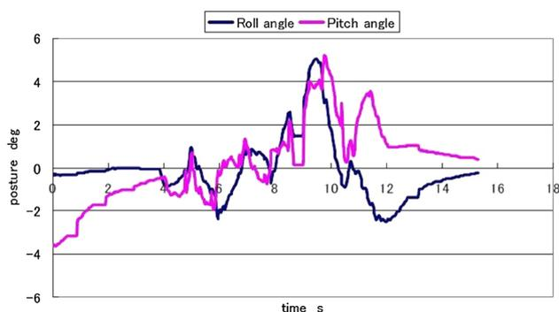
**Fig. 12** WABIAN-2R walked on the bumpy surface with tiles angled  $2^{\circ}$ – $5^{\circ}$  (forward-axis) down (experimental site no. 7)
