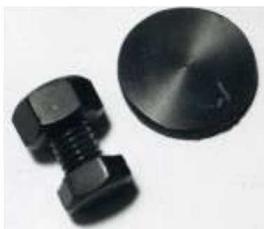
Figure 16: Machined Pieces of Polychloral
