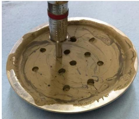
**Figure 30. Fly ash set-time test**
