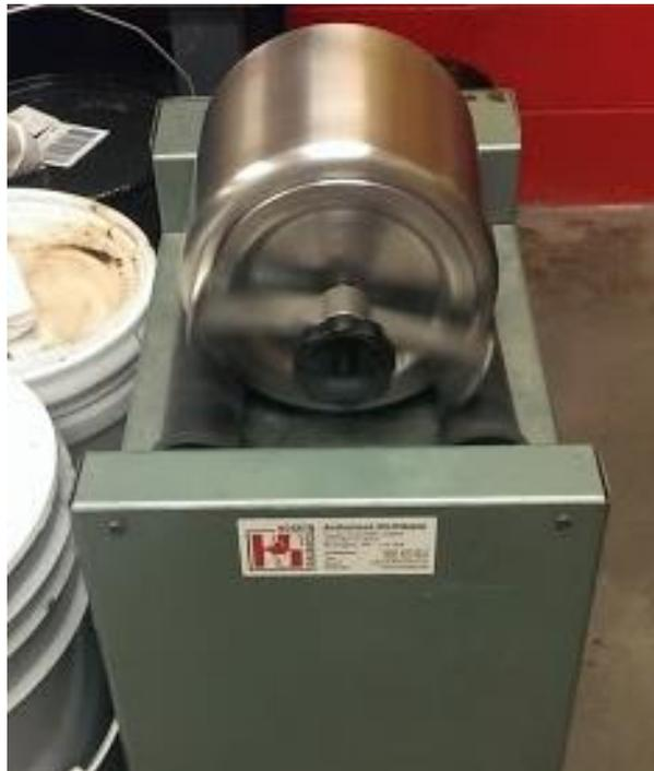
**Figure 4. Micro-Deval testing machine used in this study**
