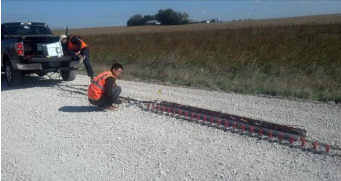
**Figure 14. MASW test setup with landstreamer**
