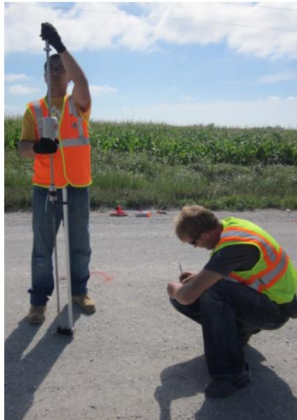
**Figure 11. Dynamic cone penetrometer (DCP) test**
