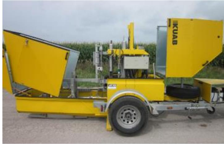
**Figure 13. Kuab falling weight deflectometer setup**
