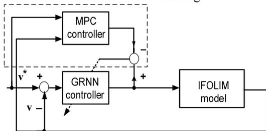
Fig. 3. GRNN control design problem based on MPC technique.
