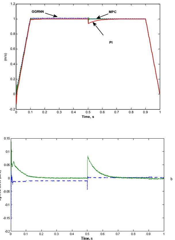
Fig. 7: a) GRNN response versus MPC and PI responses at load disturbance. b) speed error (solid line) for PI and (dashed line) for GRNN.
