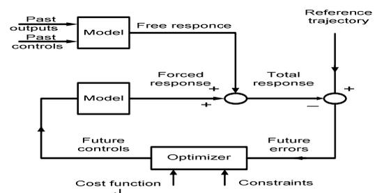
Fig. 1 A simple structure of the MPC controller.
