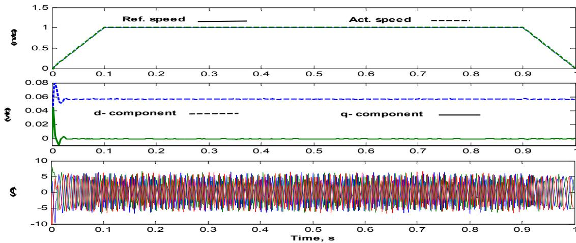
Fig. (6) Dynamic responses of the proposed system under parameters mismatch condition
