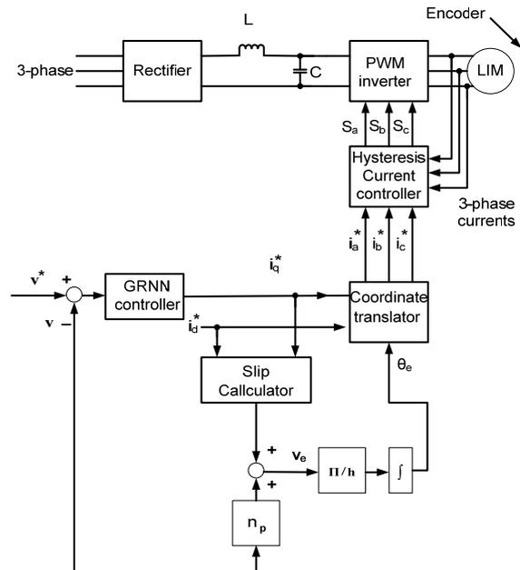
Fig. 4 Block diagram of the indirect field oriented Linear induction motor drive
