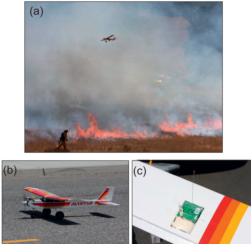
FIG. 1. (a) The miniUAS during the research flight on 7 Oct 2008, (b) completed miniUAS system during the test flight, and (c) Graw, Inc., DFM-06 radiosonde installed in the left wing of the Hobbico Avistar 40. The sensor probe extends below the wing by 10 cm allowing for good exposure to airflow.
