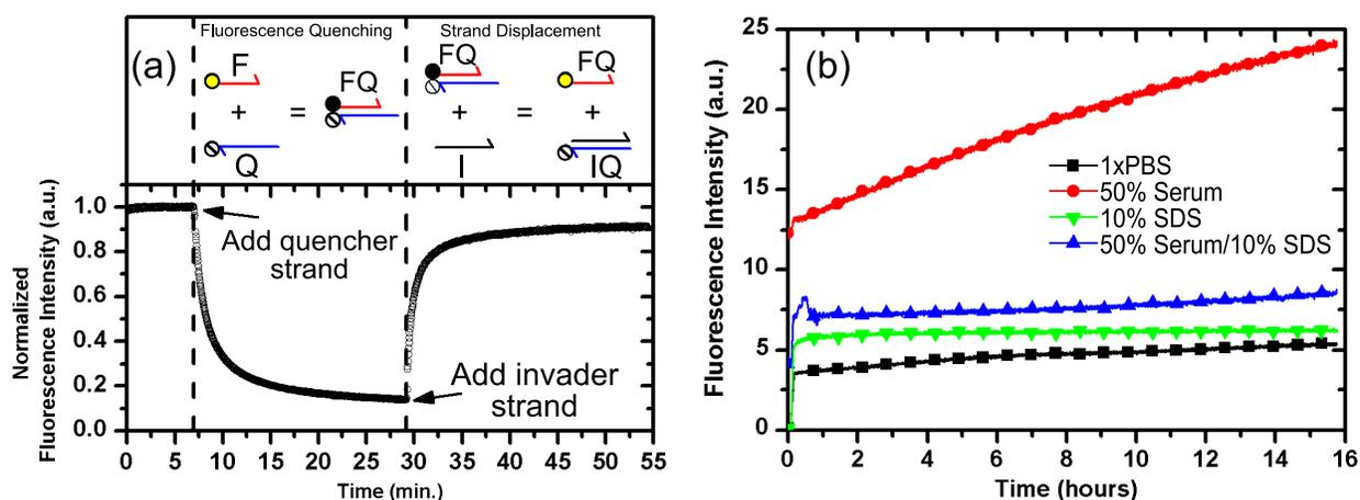
Figure 1. (a) Hybridization and strand invasion kinetics using FRET in 1xPBS. (b) Time dependent dye-quencher pair stability. The addition of 10% SDS to serum greatly increased pair lifetime.
