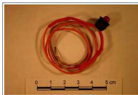
1001-60: a red Light Emitting Diode (LED) in working condition
