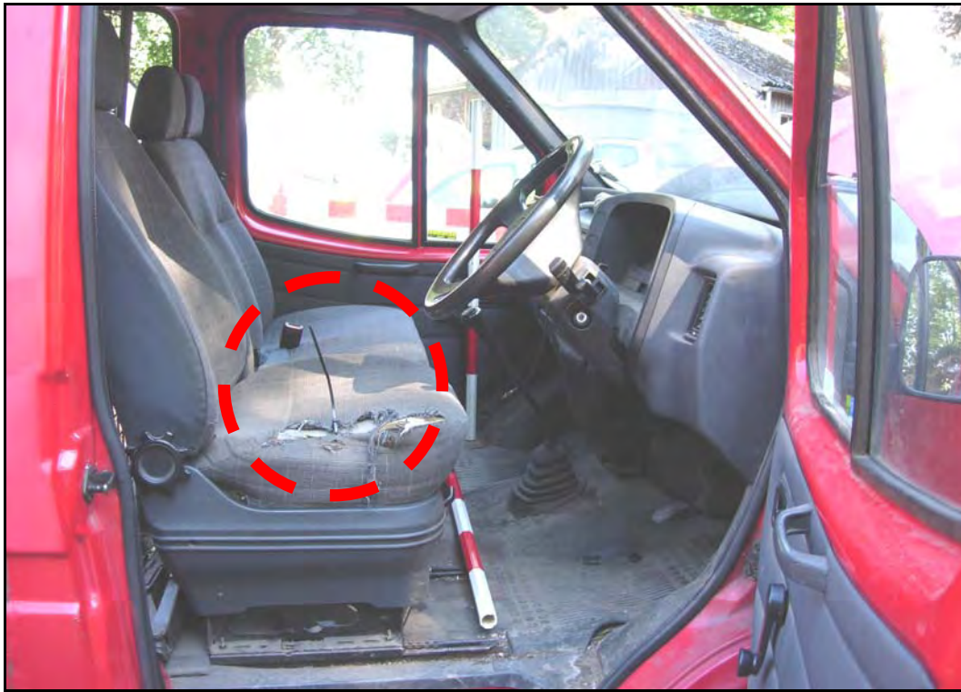
Figure 12: 'Zap Strap' seat repair (The Van Project Team)
