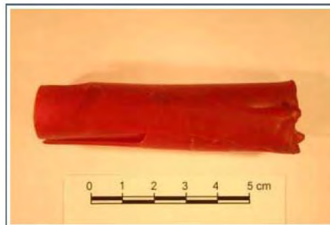
1024-3: insulation from heavy duty 'armour' electrical cable [not a shotgun shell!]
