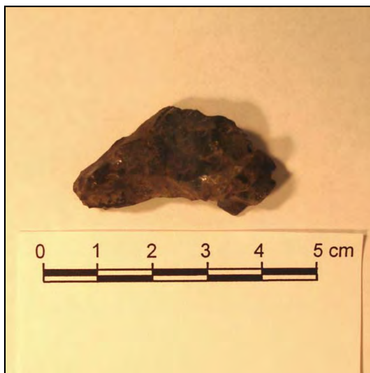
Figure 24: fragment of blast furnace slag (author)
