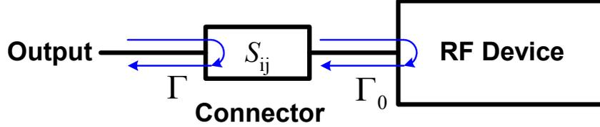
**Figure 5.** The RF connector cascade model for deriving the resultant return loss of an RF device. The single coaxial line depicting the input and output lines shown are two-port signal paths.
