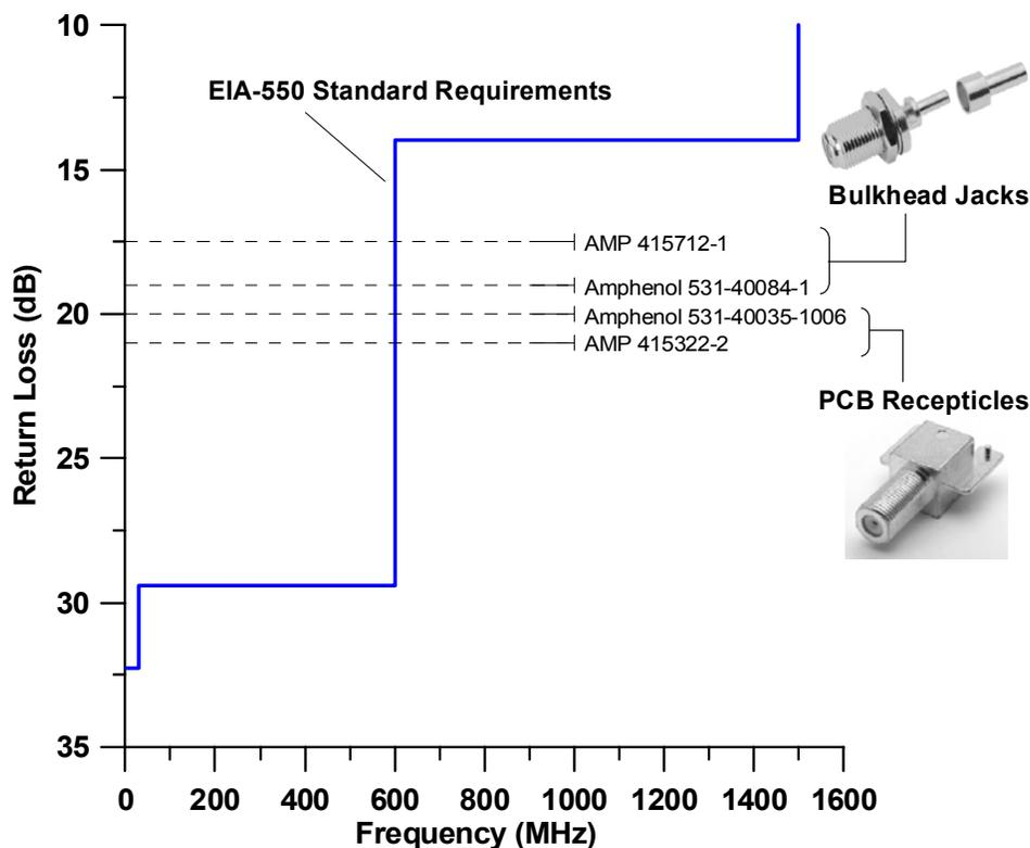
**Figure 7.** F type RF connector return loss requirements and specification limits for some commercially available connectors. To the extent that VSWR values are specified, the equivalent return loss based on Equation 25 was used. *Source:* Reference [12] for EIA-550, AMP/Tyco and Amphenol product catalogs.
