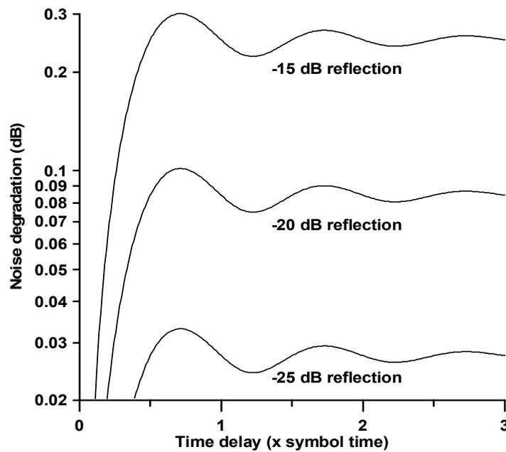
**Figure 4.** Noise degradation due to a single echo having worst case combining phase at the indicated relative reflection levels as a function delay for a QAM channel with excess bandwidth factor of  $\alpha = 0.15$ . (Based on Equation 21).
