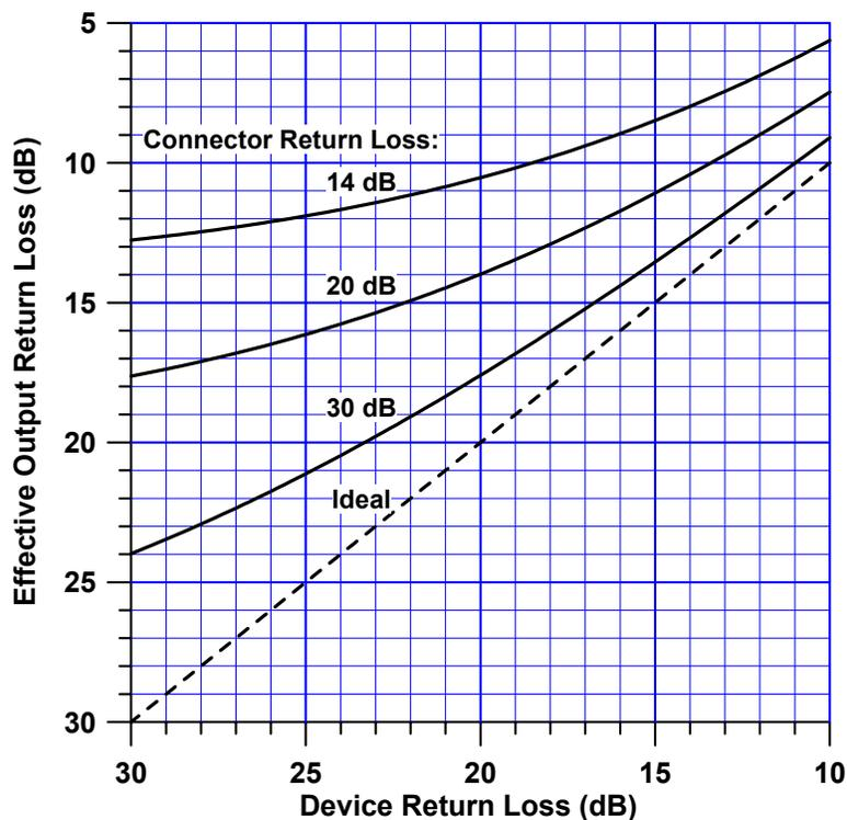
**Figure 6.** Effective output return loss degradation due to the output connector’s return loss having values of 14 dB, 20 dB, 30 dB and  $\infty$  dB (ideal). Based on Equation 24.
