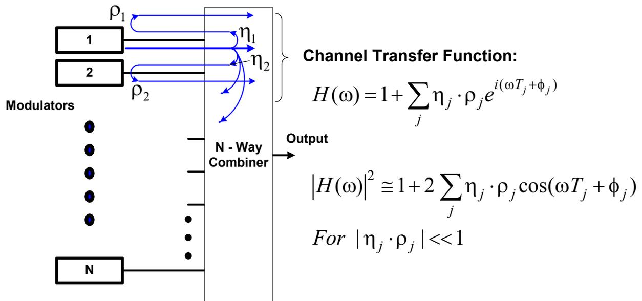
**Figure 1. Composite returns from head-end RF combiner's port reflections and modulator output returns.**
