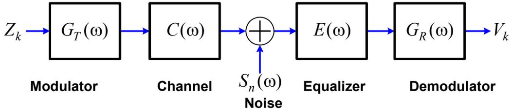
**Figure 2. Digital channel link model. The reflection distortions are subsumed within the channel transfer function  $C(\omega)$ .**
