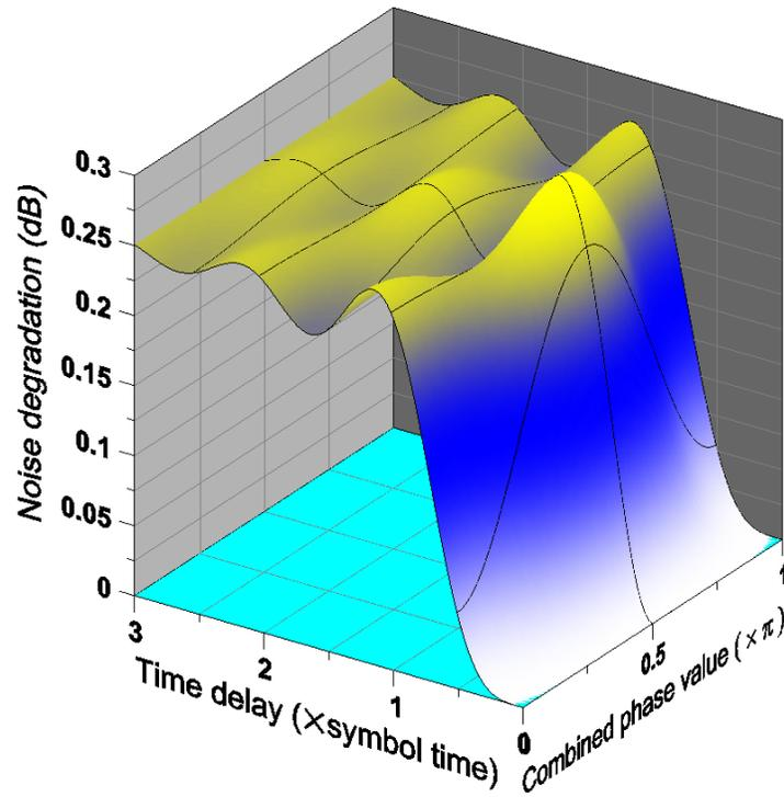
**Figure 3** Noise degradation due to a single echo having a  $-15$  dB relative level as a function of phase and delay for a QAM channel with excess bandwidth factor of  $\alpha = 0.15$ . (Based on Equation 19).
