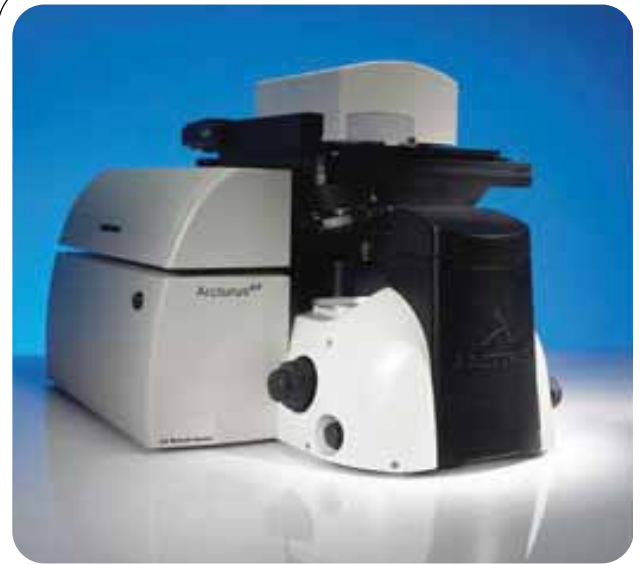
Figure 2. An example of a laser capture microscope. The Arcturus XT™ is pictured. This instrument is based on the Nikon TE2000-U inverted microscope and has both UV and IR lasers to enable both cutting and adherent laser capture microdissection. From [205].
