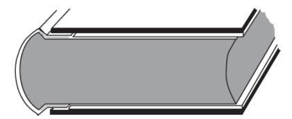
The diagram above shows how the boards are positioned next to the extensions of the spine stiffener. The head and tail turn-ins will cover these extensions where they are attached to the board, next complete the remaining turnins of the covering material.
